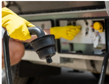
Macerator Sewage Discharge With Manual Disconnect
