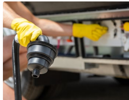
Macerator Sewage Discharge With Manual Disconnect
